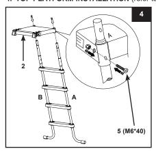
5. U-SHAPED TOP RAIL INSTALLATION (refer to figures 5.1 through 5.2): IMPORTANT: One side at a time. Do not attach the other side of the ladder until the U-shaped top rail is installed. Make sure all nuts and bolts are securely tightened. Do not fully tighten fasterners until last assembly operation.
